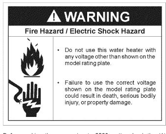
Before making the conversion to 5500 watts, check the (1) power supply . . . must be 240 volts, (2) wiring . . . 10 gauge AWG @ Type TW, 60°C or equivalent, and (3) Circuit breakers or fusing . . .capable of 30 amp loading. Also, the installation must conform with this manual, local codes and electric utility rules. Failure to comply can result in DEATH, SERIOUS BODILY INJURY, OR PROPERTY DAMAGE.
